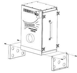
2. Use the bolts removed in Step 1 to secure Machine Mounting brackets to unit as shown in **FIG.1**.
