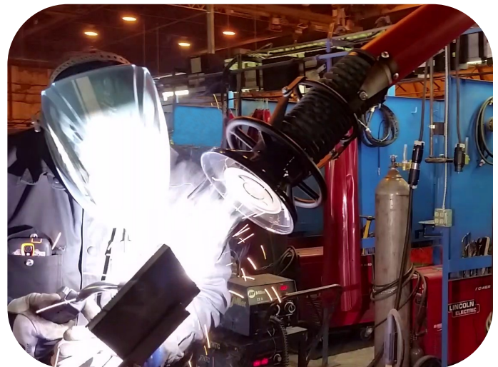
TM1000 Weld Smoke and Fume Collection
