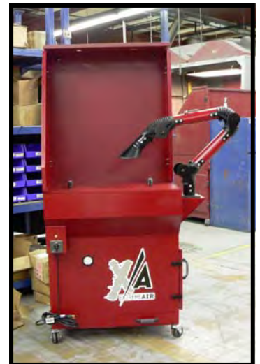
Customized Downdraft Table with 3" Overhead Source Capture Arm
