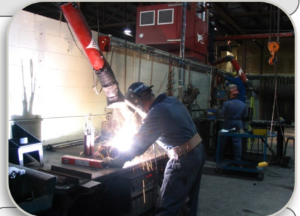
Source Capture Arms ducted to ceiling hung cartridge collector.
