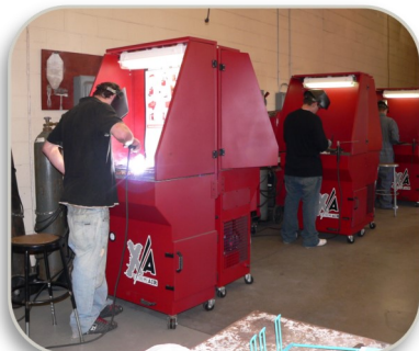
Downdraft Tables provide source capture of weld smoke and fumes.
