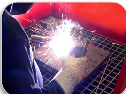
Smoke and fumes pulled away from worker breathing / vision zones.
