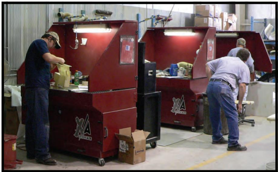
Senior Aerospace Composites is a company located in Wichita, Kansas that produces composite assemblies for the aviation industry. The customer grinds, sands, and routs composite materials in sizes varying from small to large and was looking for a way to improve the air quality in their facility and also reduce clean-up time required. The volume of dust and particulate generated was heavy and they were looking for a turnkey solution with high levels of filtration, but little to no maintenance.
