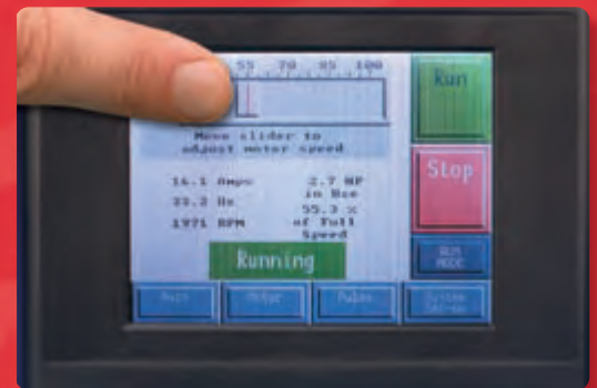
One-touch motor speed adjustment slider
