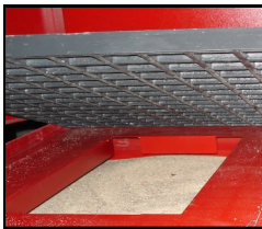
Spark Arresting Sand Trays—Standard Feature
