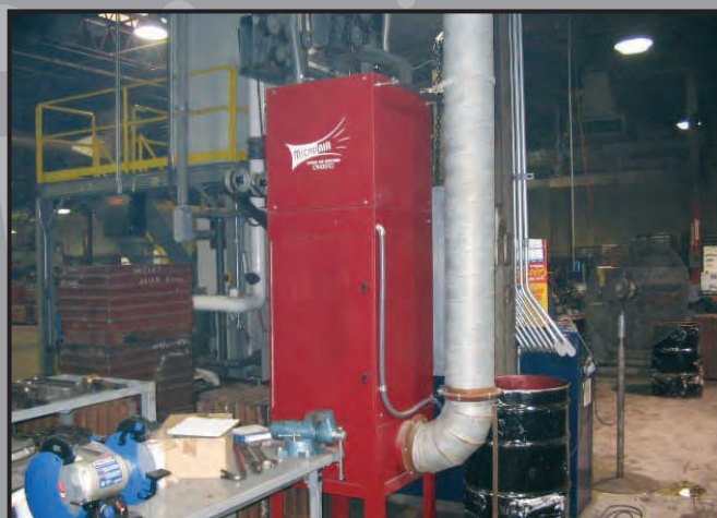
OM3510 ducted to lathe.
