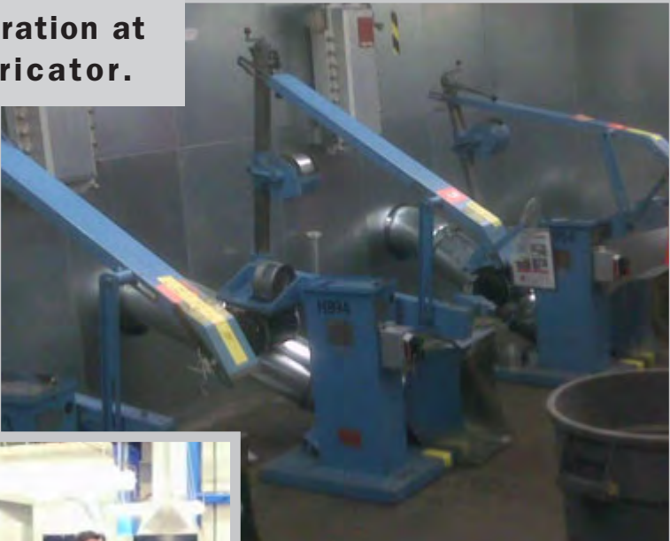
Combination of Booth Enclosures and Downdraft Tables ducted to combustible dust operations with titanium and aluminum.
