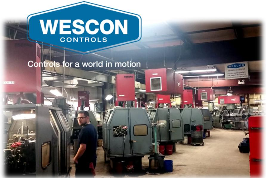
The original concept consisted of machine mounted OM550DD's for the (18) enclosed machines, and hoods ducted to OM550DD's on the (10) open machines. The machine-mounted and ducted OM550DD's would capture most of the contaminant, but, for any residual mist or haze, we suggested the addition of ambient MX3510's, configured for oil mist and equipped with carbon modules to eliminate the odors.
