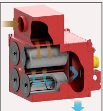
filter sections, where the contaminant is filtered and dropped into the hopper or dust drawer. Breathe Easy, clean safe air is exhausted out the bottom of the unit. Cartridge cleaning is accomplished with Micro Air's proprietary Roto-Pulse® cleaning system, where air is pulsed
