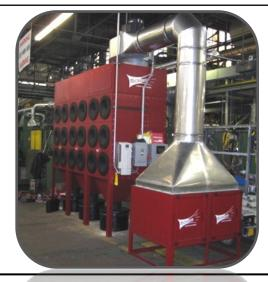
RP6-3 with Safety Filter Modules on Lead Dust Application
